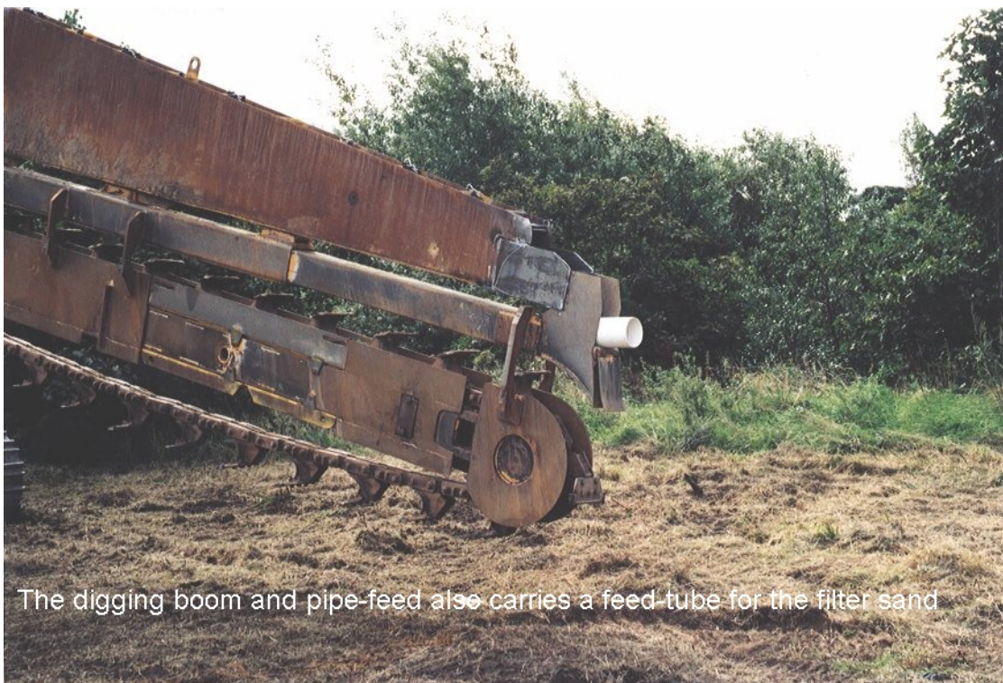
Fig 6 Detail of the cutting head
