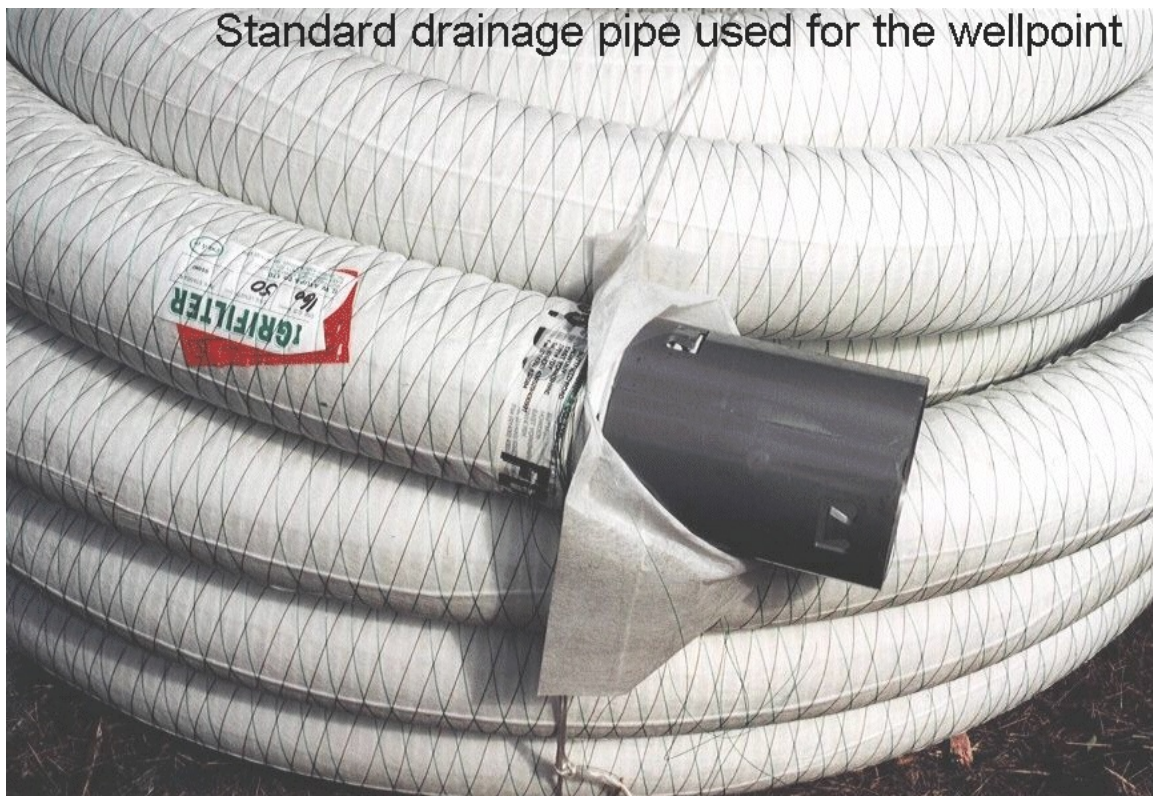
Fig 4 Coil of 150 mm diameter drainage pipe used for the HWP
