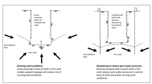
sand conditions controlled by pumped-well dewatering
